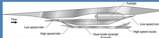
**Turbine-Based Combined Cycle (TBCC) Engine**
