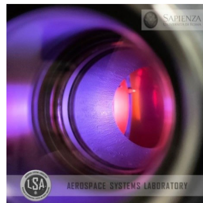
Carbon/Carbon plate subjected to Atox and UV irradiation
