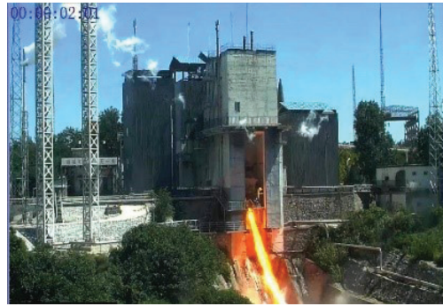
Test of the LOX-LH2 engine for the 3rd stage of Long March 9
