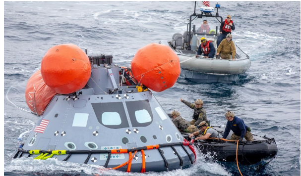
U.S. Navy divers from Explosive Ordnance Disposal (EOD) Expeditionary Support Unit 1, attach tending lines to a mock Orion capsule during Day 2 of Underway Recovery Test 9 (URT-9) aboard the USS John P. Murtha. During the weeklong test, NASA's Landing and Recovery team completed their final mission certification ahead of Artemis I.
