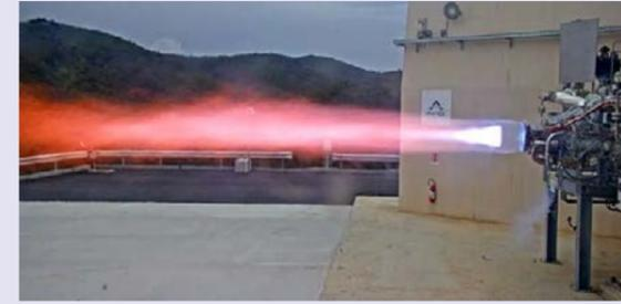
Firing test of the M10 engine (courtesy AVIO S.p.A.)
