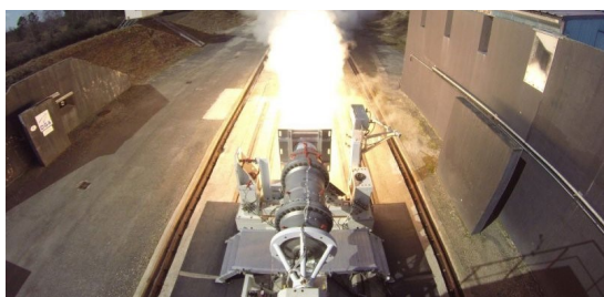
M4R2 VINCI® engine mounted in the new test cell PF52 (Vernon, France)
