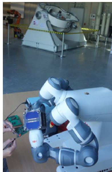
Human-robot cooperation in integration of satellites. Turntable test equipment for simulation of dynamics in the background
