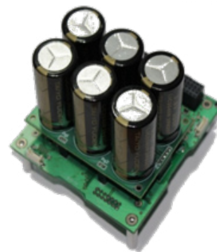
Figure 5: NART-EPS with Super-Capacitors
