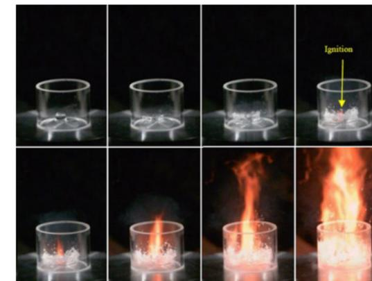
The propellant developed at Łukasiewicz – ILOT is a safer alternative for personnel and the environment to the toxic materials currently in use – hydrazine derivatives and nitrogen oxides. The developed combination uses hydrogen peroxide (with a concentration of 98%) as oxidizer with a novel fuel.
