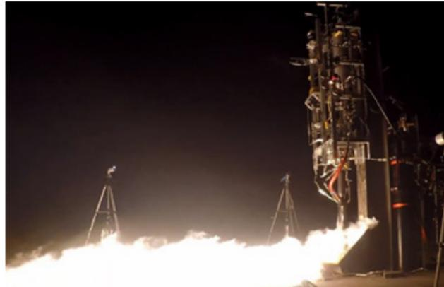
This was the LPL's first successful test fire of a regeneratively-cooled engine and one of the few successful ones to date in collegiate rocketry. The student group additively manufactured this engine by laser powder bed fusion with the help of its industrial partner i3DMFG. LPL will test-fire this engine again later this year, introducing adding important thrust vectoring capability.
