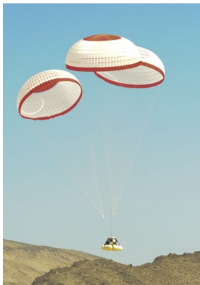
Final drop test for Boeing's CST-100 spacecraft at an altitude of 4.3 km Credit: Elizabeth Morrell/Boeing
