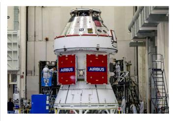
Airbus ESM, connected to the crew module via an adapter to form the Orion composite ©NASA
