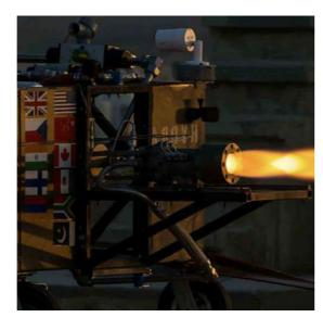
The Viterbi School of Engineering's Liquid Propulsion Laboratory (LPL) at the University of Southern California designs, builds, and tests industry-grade liquid rocket engines and feed systems.
