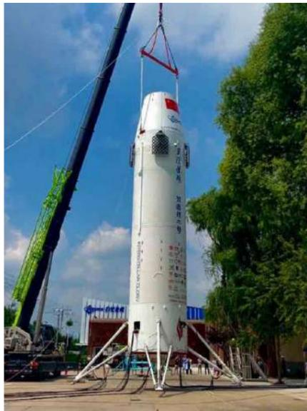
The complete success of the whole body drop test of Hyperbola-2Y (SQX-2Y) reusable liquid launch vehicle marks one more major breakthrough in the field of reusable rocket achieved by Interstellar Glory, providing solid foundation for subsequent flight tests of the reusable launch vehicles.
